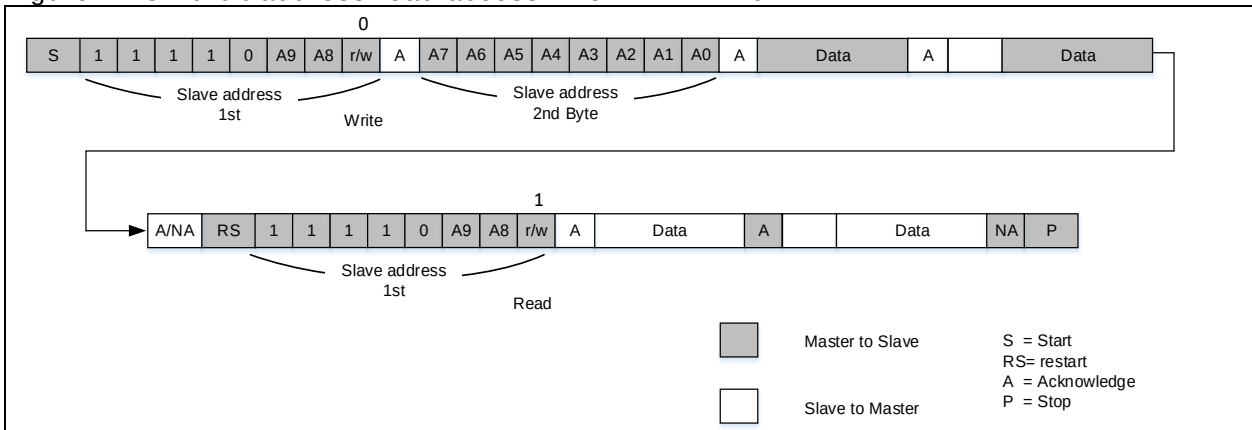
Figure 11-9 10-bit address read access when READH10=0
